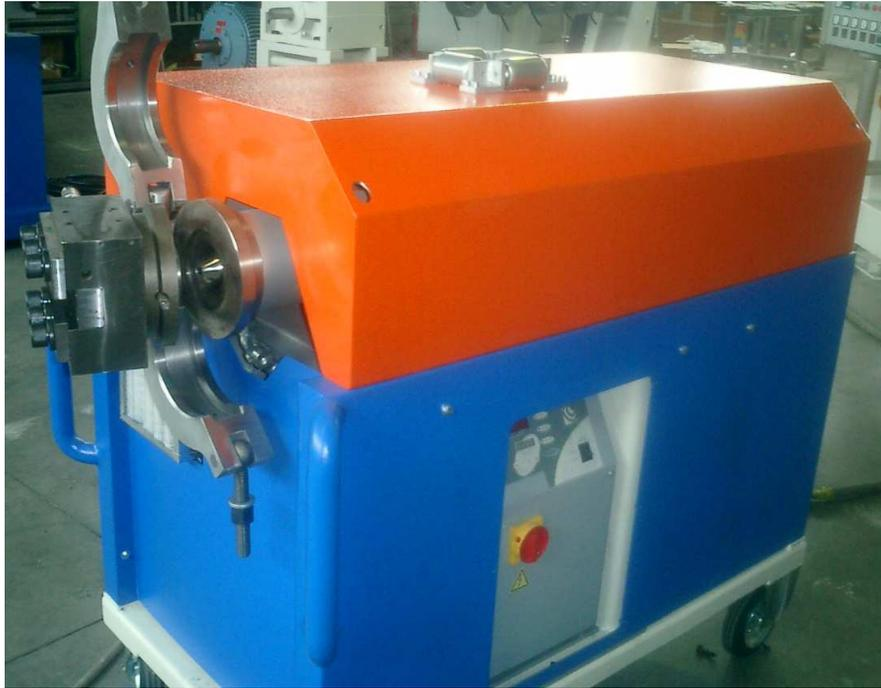
**Extruder mounted on wheels for easy positioning**
